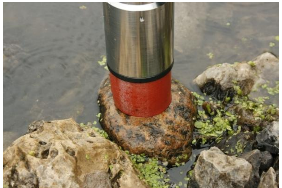
bbe BenthoTorch: for measurement of benthic algae on different substrates
