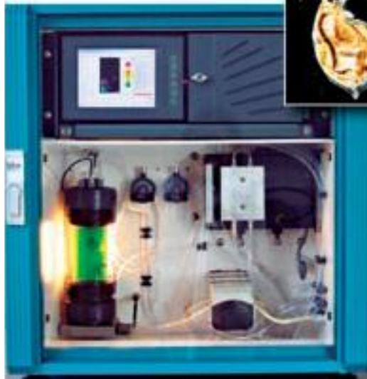
A biomonitor continuously monitors the swimming speed and behavior of Daphnia water fleas (inset photo). Significantly abnormal behavior indicates water contamination and triggers an alarm.
