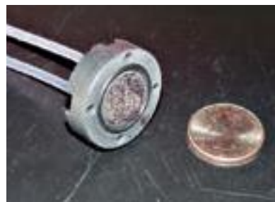
In a big step for little devices, this miniature microbial fuel cell produces remarkably high power levels. The spaghetti-like 3D graphite felt electrode visible inside the chamber is the key to its power.
