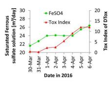
An increased use of ferrous sulfate as flocking agent for phosphate is suspected as the cause for the rising toxicity index of the Daphnia-Toximeter (s. left diagram).
