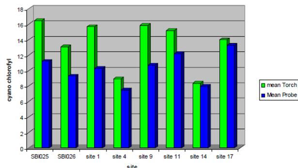
Figure: Comparison of AlgaeTorch in situ and FluoroProbe laboratory analysis
