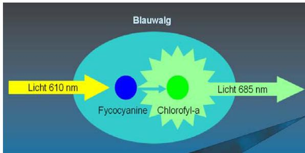
The experiments for the investigation were carried out using the FluoroProbe II by bbe Moldaenke GmbH. The robustness of the fluorescence analysis (linearity and repeatability) was very good. There was a significant linear relationship with chlorophyll determined by the Dutch NEN 6520 method. This can be used to compare the method with other instruments
