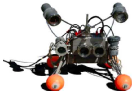
REMOS1 3D in-situ imaging system (Fish)
