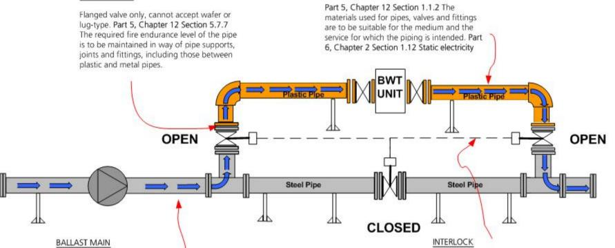
Part 6, Chapter 2 Section 1.5 Essential services are those necessary for the propulsion and safety of the ship, Ballast pumps are included. Materials sensitive to heat are not to be used in piping systems essential to the safe operation of the ship, or containing seawater where leakage or failure could result in fire or in flooding.
