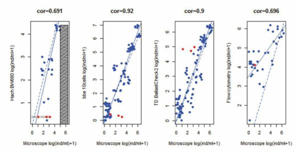
The red dots show the UV-treated samples. The low detection limit and the sophisticated measuring principle of the 10cells enable the user to analyse ballast water quick and easy at the requested mesaurement range.
