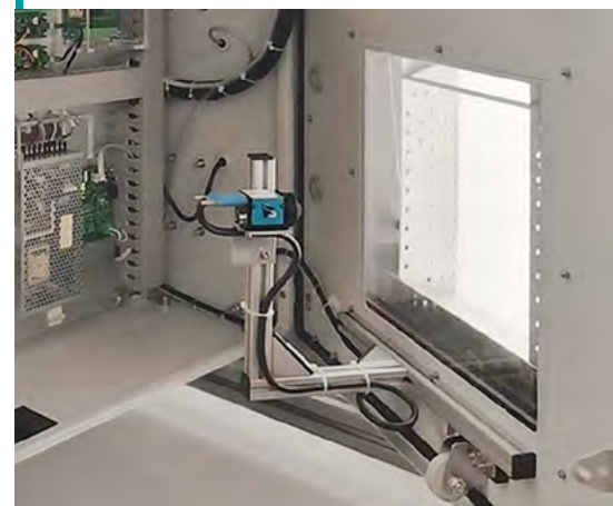
The behavior of the fish is permanently monitored with a USB camera
