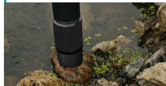
The BenthoTorch used to measure algal classes and their concentration on a stone surface.
