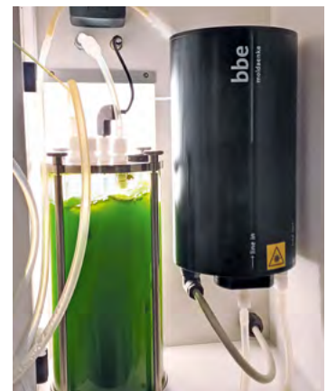
Sample water is mixed with the algae test solution and then analysed.
