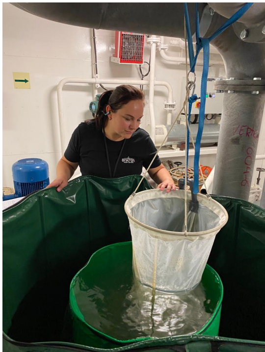
Figure 3: Sampling process for ballast water.
